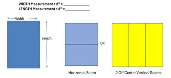
A Horizontal seam is always my preference – it lays nice and flat/smooth along the take up roller – instead of building up(4 layers at a time) in the center with every turn of the bar – which can cause saggy outside edges. (2 off center vertical seams are better than one center vertical seam)
